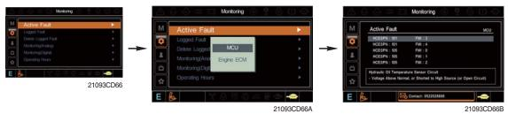
$\cdot\,$  The active faults of the MCU or engine ECM can be checked by this menu.
